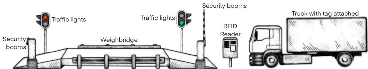
The vehicle driver will approach the RFID reader, which will automatically scan the attached RFID tag. If the tag's details are invalid or if the vehicle has been barred from the system, the security booms and traffic lights will remain unchanged, preventing the vehicle from proceeding.
