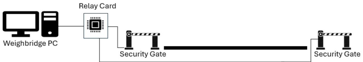
The **W8Link Relay Station** enables the **W8Suite** Module to interface with a relay card, facilitating the automation of traffic lights, sensor beams, and security gates based on events within the W8Suite module.
