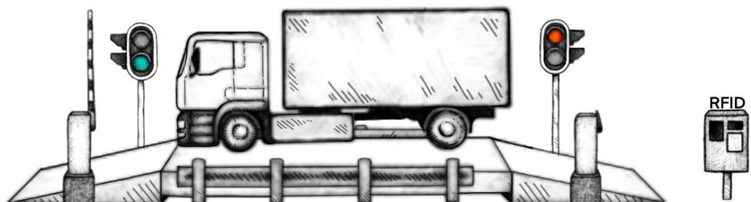
When the driver exits the weighbridge and the vehicle's weight is no longer detected, the security booms will close, and the traffic lights will turn red, as illustrated below. At this point, the weighbridge is ready for the next weighing transaction.
