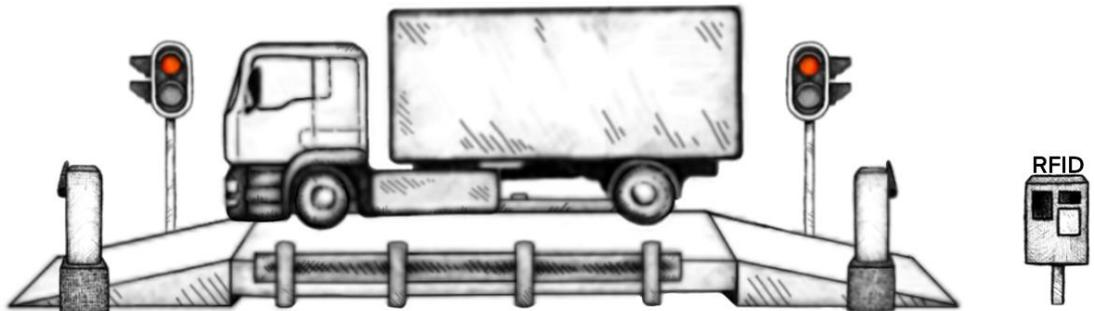
Once the process has been completed in the background, the security booms will open, and the traffic lights will turn green, indicating that the transaction has been successfully processed. This signals to the driver that they are free to exit the weighbridge. Please refer to the illustration below for a visual representation.
