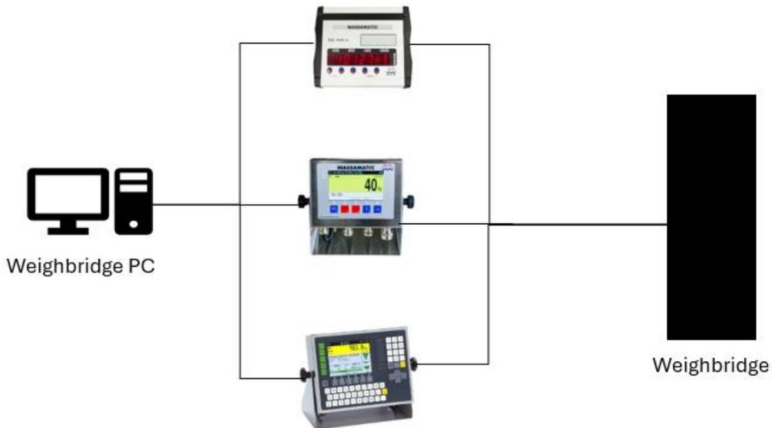
The primary function of the **W8Link Weigh Station** is to read various data strings from multiple indicators. A single W8Link: Weigh Station can interface with multiple indicators connected to a PC, as illustrated.
