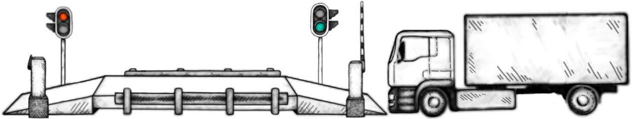
The driver will then proceed to drive the vehicle onto the weighbridge. Once the truck is correctly positioned on the weighbridge, the security booms will close, and the traffic lights will turn red, signalling that the vehicle is securely stationed, as shown in the illustration below.
