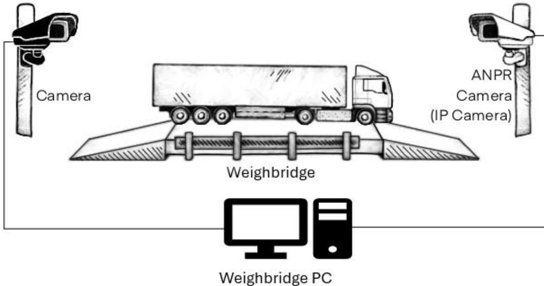
The **W8Link Camera Station** is designed to capture images from cameras based on various events configured in the W8Suite Module. For example, it can take a picture of a vehicle before a weighing transaction or while the vehicle is on the weighbridge during a transaction. These images are then associated with the transaction for easy access and future reference.
